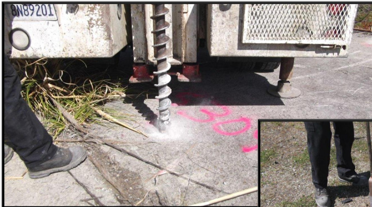
Direct push sampling through concrete foundation
